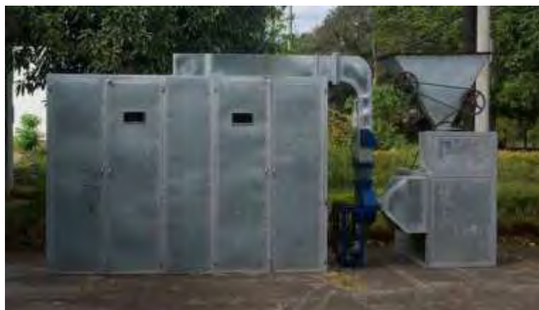
The rice husk-fuelled cabinet dryer FD-200
