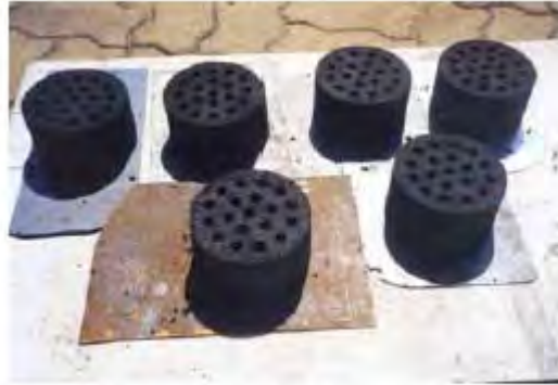
Figure 7.7: Drying of molded honeycomb briquettes
