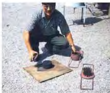
Figure 7.6: Briquette-making using the mould
